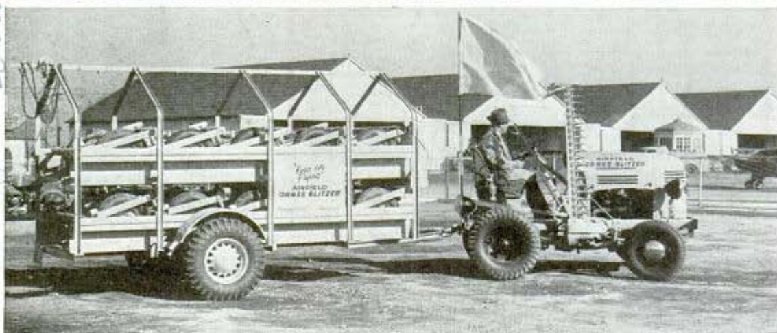
Tractor, top, tows the nine cutting units; bottom, cutters loaded on trailer for trip over highway
